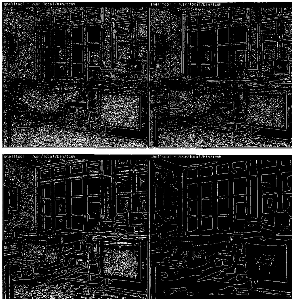
Fig. 15. Multiscale edge detection using the recursive Laplacian. Upper left: Zero-crossings with \alpha = 1 . Upper right: Zero-crossings with \alpha = 0.75 . Lower left: Zero-crossings with \alpha = 0.5 . Lower right: Zero-crossings with \alpha = 0.25 .
