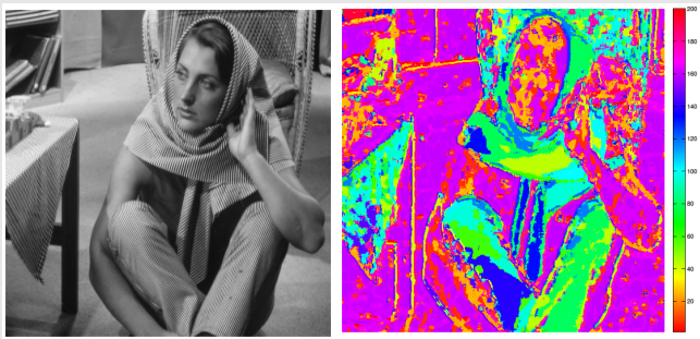
Figure: Denoising of an image using GMM: on the left original image, on the right the color code represents the chosen GMM. Similar textures are represented by the same model.
