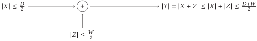
Fig. 6. The uniform aiming channel under amplitude constraint.
