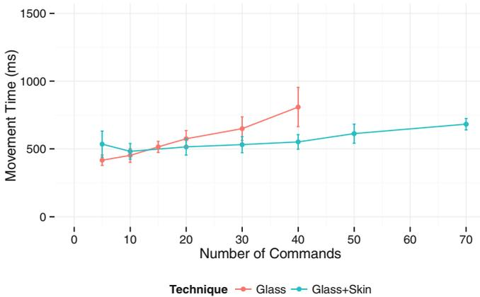
**Fig. 4.** Mean *MT* vs. the number of commands for each condition.
