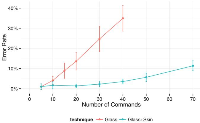
**Fig. 6.** Error rate vs. the number of commands for each condition.
