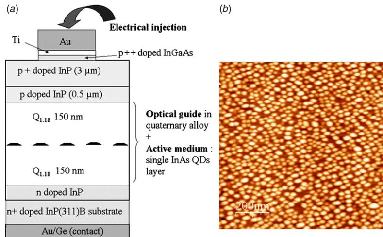
**Figure 1.** (a) Schematic drawing of the InAs/InP laser structure containing a single InAs QD layer. (b) AFM image of an uncapped QD layer: an average diameter of 30 nm could be deduced, along with an average height of 3 nm. The QD density was evaluated to be above  $10^{11} \text{ cm}^{-2}$ .
