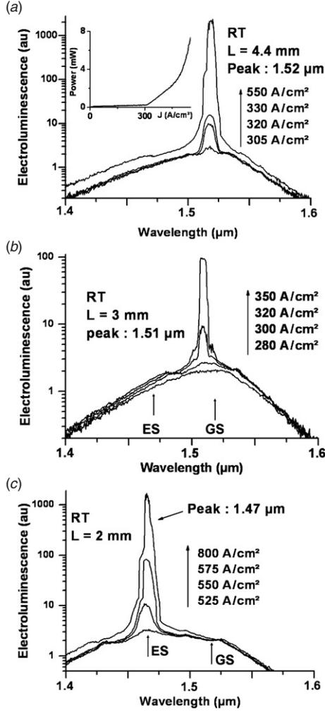
**Figure 3.** Electroluminescence spectra obtained at room temperature, for (a) the 4.4 mm, (b) the 3 mm and (c) the 2 mm cavity length devices. In the inset in figure 3(a) is given the light–current curve for the longer device.
