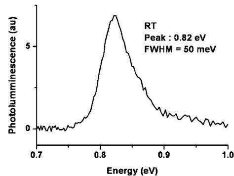
**Figure 2.** Photoluminescence spectrum of the epitaxied structure. The graph shows a peak at 0.82 eV (corresponding to a  $1.52 \mu\text{m}$  wavelength), and a FWHM of 50 meV (91 nm). This low FWHM can be explained by the reduced QD size dispersion due to optimized growth techniques.
