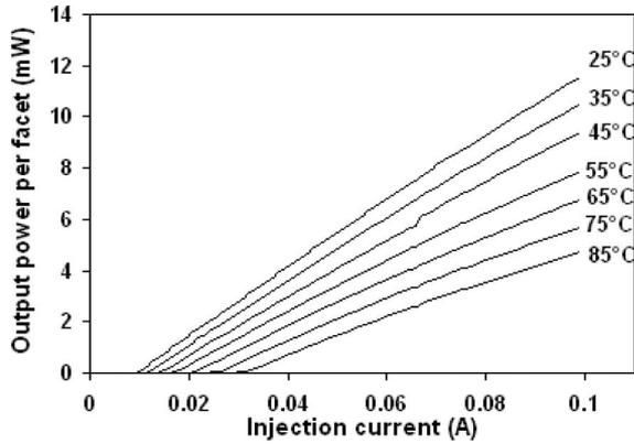
Fig. 4. Light-current characteristic of a quantum-dash-based laser as a function of the temperature.
