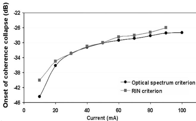
Fig. 2. Onset of CC, determined both from the optical spectrum and the RIN, of a 205- $\mu\text{m}$ - long DFB quantum-dash-based laser versus the injection current. Reprinted with permission from [12].
