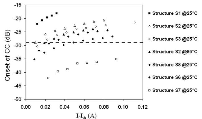
Fig. 10. Onset of CC of  $600\text{-}\mu\text{m}$ -long quantum-dash-based lasers (the dashed line represents the minimum value required for isolator-free operation).
