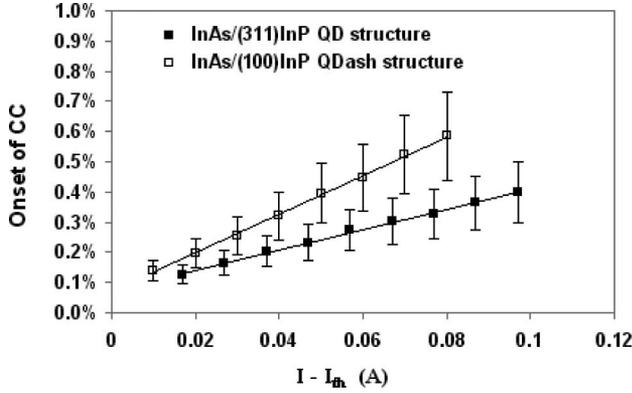
Fig. 11. Onset of CC as a function of the current difference for a 1100- $\mu\text{m}$ -long quantum-dot-based laser and for a 1200- $\mu\text{m}$ -long quantum-dash-based laser.
