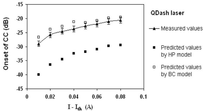
Fig. 12. Comparison of experimental data with predicted values for a quantum-dash-based laser (structure S2).
