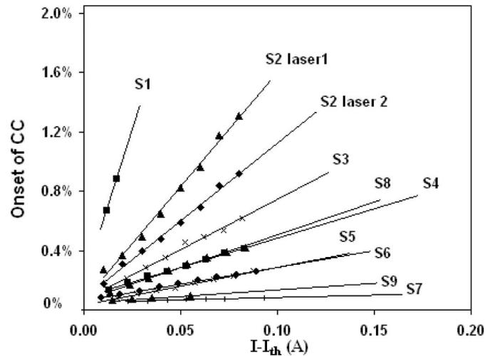
Fig. 3. Onset of CC of several 600  $\mu\text{m}$ -long Fabry–Perot quantum-dash-based lasers as a function of the current difference. Reprinted with permission from [23].
