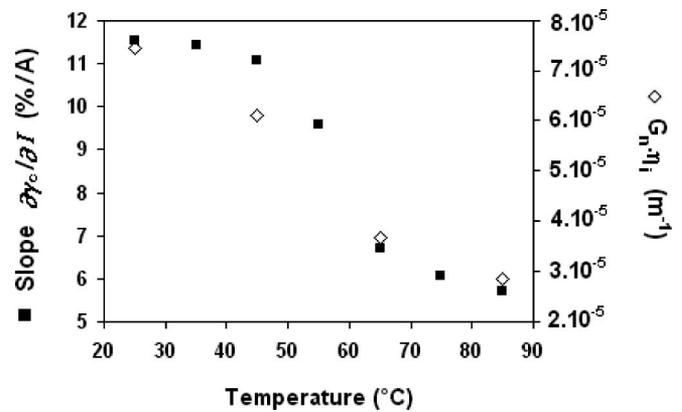
Fig. 6. Parameter  $G_n\eta_i$  and slope  $\partial\gamma_c/\partial I$  versus temperature.
