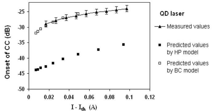
Fig. 13. Comparison of experimental data with predicted values for a quantum-dot-based laser.
