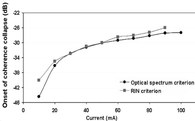
Fig. 2. Onset of CC, determined both from the optical spectrum and the RIN, of a 205- $\mu\text{m}$ -long DFB quantum-dash-based laser versus the injection current. Reprinted with permission from [12].
