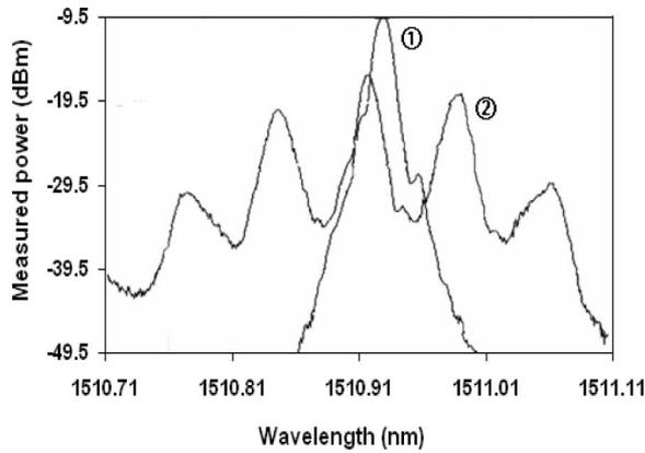
Fig. 1. Optical spectrum: (1) without optical feedback; (2) with optical feedback and onset of CC Reprinted with permission from [12].
