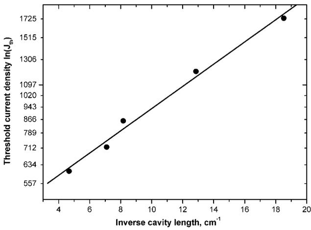
**Fig. 3**  $\ln J_{th}$  (log scale) versus  $1/L$  for InAs/InP broad-area lasers of  $50 \mu\text{m}$  width and cavity lengths ranging from  $\sim 800$  to  $1800 \mu\text{m}$
