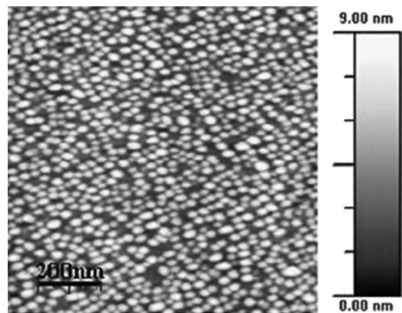
Fig. 1 Atomic force microscopic view of a dot layer
