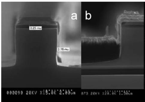
**Fig. 5** SEM view of a ridge on InP(3 1 1)B
