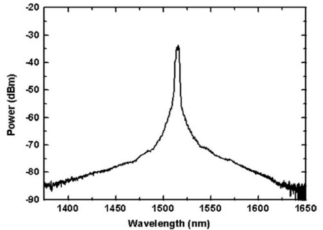
**Fig. 7** CW room temperature optical spectrum of a  $1490 \mu\text{m} \times 2.5 \mu\text{m}$  ridge laser measured ( $I = 1.85 I_{th} \approx 111 \text{ mA}$ )
