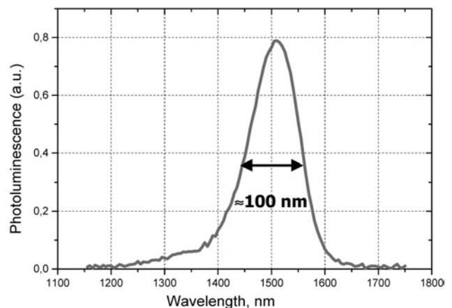
Fig. 2 PL spectrum at room temperature, FWHM = 58 meV
