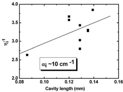
**Fig. 4** Inverse external efficiency as a function of cavity length
