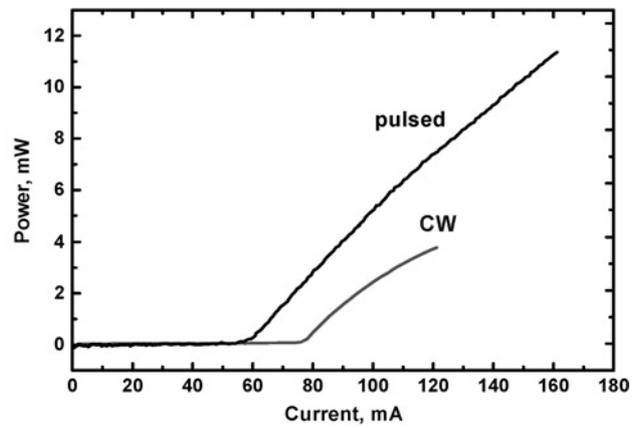
**Fig. 6** Light-current characteristic of a  $1490 \mu\text{m} \times 2.5 \mu\text{m}$  ridge laser measured under pulsed and CW operations at room temperature
