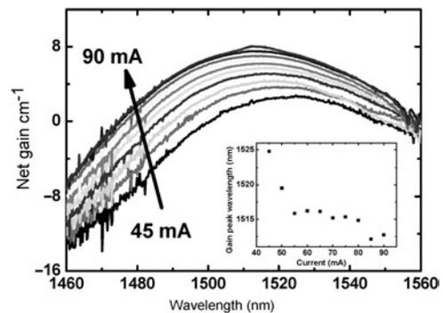
**Fig. 8** Net gain spectra in CW regime for current increasing from  $45$  to  $80 \text{ mA}$  ( $L = 1490 \mu\text{m}$ , threshold current equals  $80 \text{ mA}$ )
