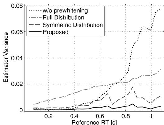
**Fig. 5.** Variance of the estimator when the prewhitening stage is ignored (dotted), when the whole decay rate distribution is considered (dash-dotted), when the symmetric distribution is used (dashed) and using the truncated distribution and the prewhitening stage as described above (solid).
