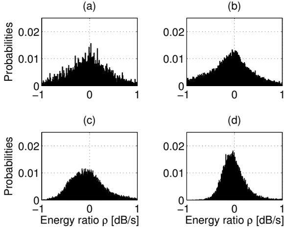
**Fig. 1.** Distribution of the energy ratios for some RT values: a) Anechoic speech, b)  $RT = 250$  ms, c)  $RT = 500$  ms and d)  $RT = 1$  s.
