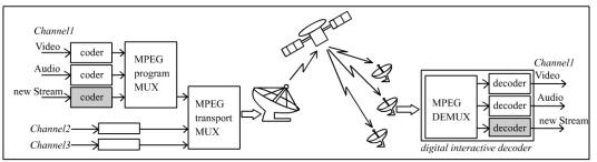
Figure 1: typical transmission chain of broadcast interactive channels
