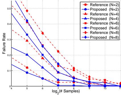
**Fig. 1.** Comparison between the reference and the proposed technique for finite field  $\text{GF}(2)$ . The failure rate, *i.e.*, the percentage of sources that the algorithm was not able to identify, is plotted against the number of samples in the mixture in log-scale.
