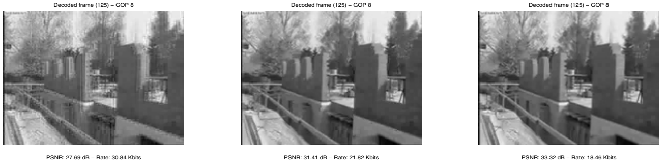
Fig. 6. Visual results comparisons between the proposed algorithms (alg. 1 - center, and alg. 2 - right) and DISCOVER codec (left) for the decoded frame 125 of Foreman sequence for GOP size 8.
