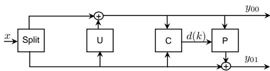
**Fig. 2:** Adaptive prediction lifting scheme
