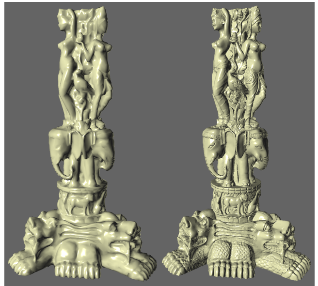
(b) XYZRGB Statue, original mesh has 10M triangles, the simplified one 20K. Texture dimension: 4096x3705
