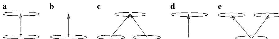
FIG. 5. The matching relations between gray-level blobs through the scales: (a) plain link, (b) annihilation, (c) merge, (d) creation, (e) split.
