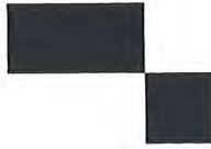
Figure 11: Definition 14 reduces to the binary definition in the crisp case. The degree of adjacency between the black boxes is equal to 1 if we use 8-connectivity, and equal to 0 if we use 4-connectivity.
