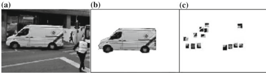
Fig. 4 Two ways to extensionally describe the vehicle in figure a : b by a mask that specifies the object pixels, c by a list of patches around points of interest
