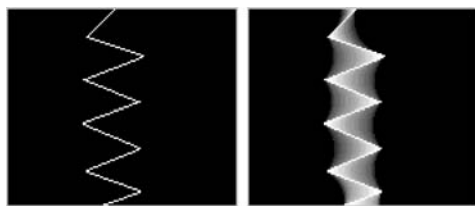
Figure 22. Viscous closing of a synthetic image. The original contour is a one pixel thin line. The viscous closing gradually thickens the contour.
