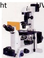
Resolution is limited to approx. 1/2 the wavelength of illuminating source
