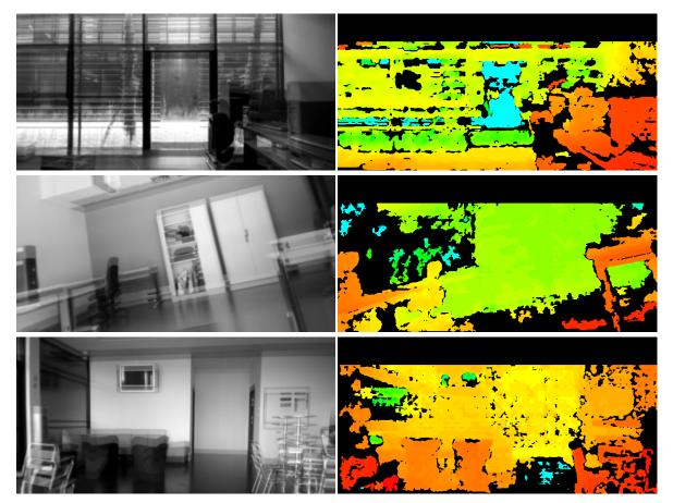
Figure 9: Dense 3D reconstruction results: The overlayed rectified images before and after the height change visualize the precision of the estimated camera motion (left). Therefore, any standard implementation for distance reconstruction, e.g. [11], may be used without modification (right).
