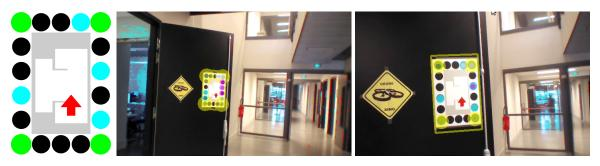
Figure 10: Landmark with machine-readable dot pattern and human-readable floor plan (left). Approach towards a detected yet un-recognized landmark (middle). Recognized landmark just before re-orientation for further flight (right).
