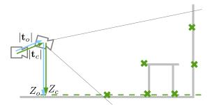
Figure 3: The ground plane is correctly identified by the 4<sup>th</sup> step of sparse 3D reconstruction. The camera's height  $Z_c$  above it may safely be assumed to equal the altitude  $Z_o$  measured by the on-board ultrasonic sensor.
