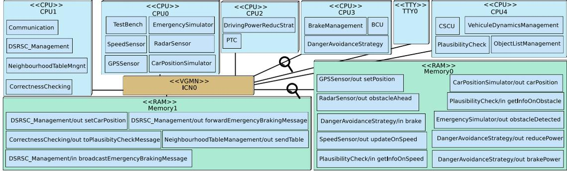
Fig. 4. Deployment Diagram of the Active Braking Application: five CPUs and two RAMs
