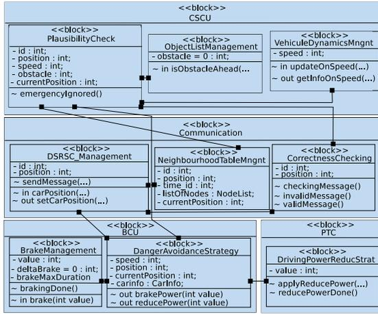
Fig. 3. Active Braking Block Diagram
