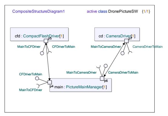
The composite structure diagram is the one of *DronePictureSW*. It shows only internal ports.
