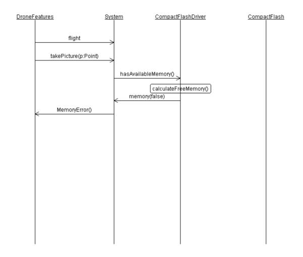
In this error scenario, one can notice that the hardware part of the CompactFlash system is not involved in the free memory management.
