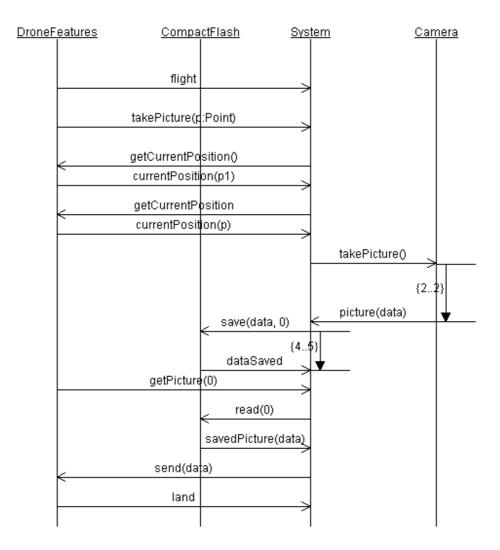
On this scenario, we show a regular trace that consists first in the activation of the picture management (flight message), then, in taking a picture. Then, the picture is saved on card. When requested, data are first fetched from card, and then transferred to the drone. Once the drone has landed, picture management is no more functional. Also, this scenario doesn't show what happens if several concurrent orders are received: this issue is addressed at state machines diagrams level.
