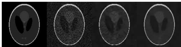
Fig. 3. From left to right: synthetic 128 \times 128 phantom image; noisy image (MSE=739); PDE scheme (MSE=305); nonlocal scheme (MSE=299).
