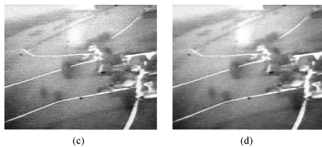
Fig. 9. Aircraft navigation images, SNR = 8 dB: (a) LLTV image (b) FLIR image (c) Fused image: Least square (d) Fused image: Proposed approach.
