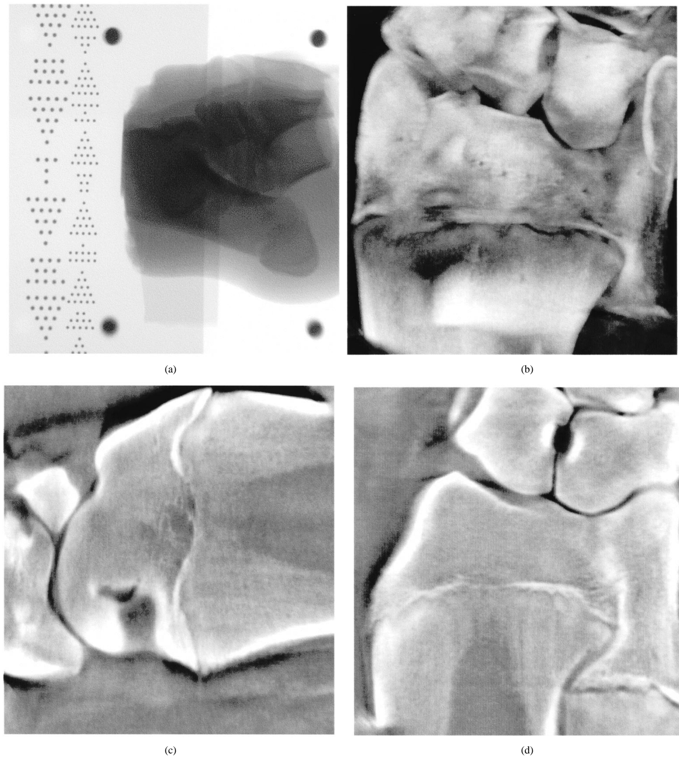
Fig. 11. Bone imaging with a joint of a cow's leg. (a) One selected original projection of the object together with the marker ring for pose determination. (b) y -MIP of the reconstructed 3-D VOI. (c) Selected x -slice through the reconstructed volume. (d) Selected y -slice through the reconstructed volume. Voxel size: 0.38 mm, 100 projections.
