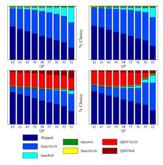
Fig. 6. Mode distribution,  $16 \times 16$  and  $8 \times 8$  enabled, for the sequence *Tempete*. First row: H.264 at 1/4-pel, H.264 at 1/8-pel, second row: QMV "Oracle," QMV "Minsum."
