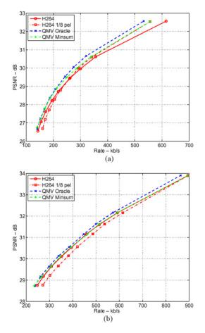
Fig. 8. Rate-distortion performance of the QMV coding mode, SD sequences. (a) *City* SD at 30 frames/s. (b) *Soccer* SD at 30 frames/s.
