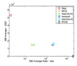
Fig. 5. Operation points with the new QMV 16×16 mode, sequence City.
