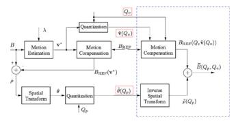
Fig. 2. New coding mode: quantization of motion vectors. In red: the information that the encoder sends to the decoder. The dashed box represents the decoder. The reference information  $B_{REF}$  is known both by the encoder and the decoder.
