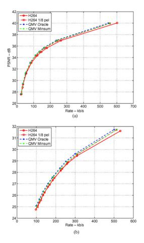
Fig. 7. Rate-distortion performance of the QMV coding mode, CIF sequences. (a) *Container CIF* at 30 frames/s. (b) *Tempete CIF* at 30 frames/s.
