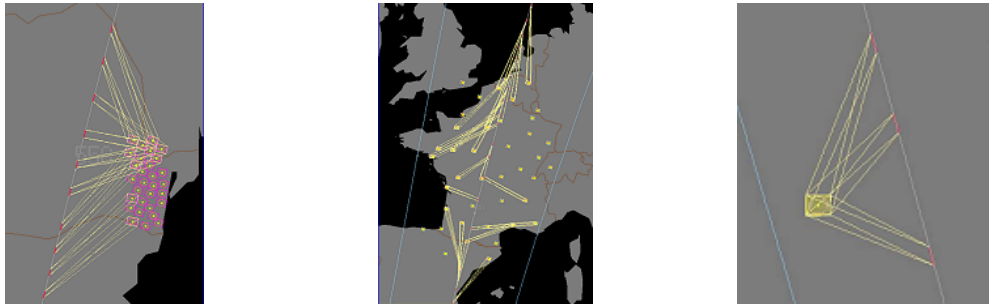
Figure 1.3: PLEIADES capabilities (from left to right) : adjacent regions, disjoint regions, tri-stereoscopic acquisition.
