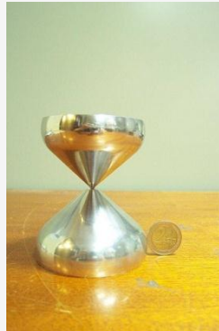
An instrumentation antenna (for channel measurements)
