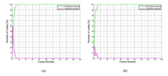
Figure 1. (a) Received frames for 60 nodes in  $76 \times 76$  m<sup>2</sup>. (b) Received frames for 180 nodes in  $132 \times 132$  m<sup>2</sup>.
