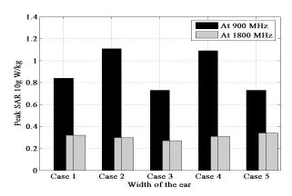
Fig. 5. Peak SAR over 10g using a handset
