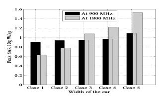
Fig. 6. Peak SAR over 10g using a dipole
