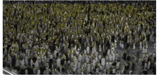
Fig. 2: Example of detection results of the RetinaNet, with ResNet-50 as architecture. Multiple factors such as the density, occlusion level and homogeneity of the scene impede significantly the tracking process.
