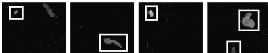
Fig. 4. Temporal detections of blotches, corresponding to the images in Fig. 1. White boxes show examples of semi-transparent and opaque blotches well detected, while remaining detections are caused by pathological motion.
