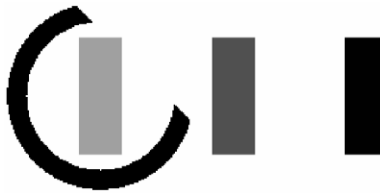
Fig. 14. An example of a concave reference object and a rectangle having an increasing distance to it.
