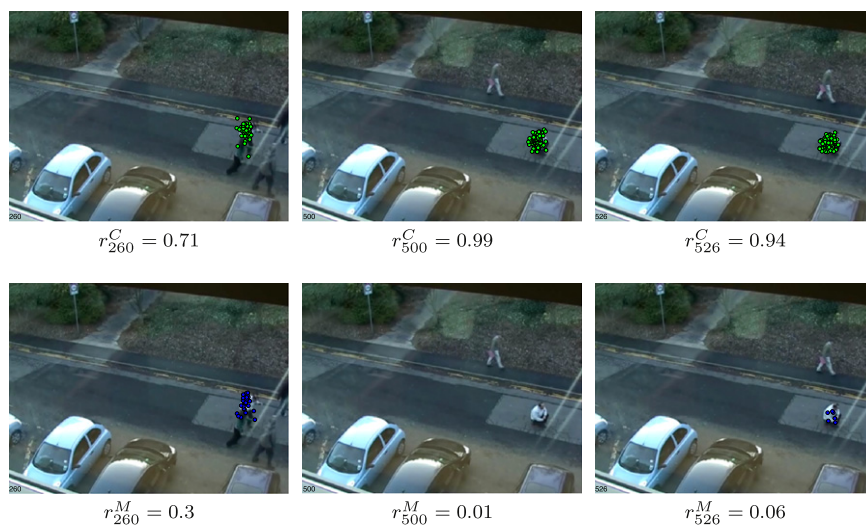
Fig. 3. Seq. 1 Visual representation of the cue reliabilities at three sample frames (green for color and blue for motion). (For interpretation of the references to color in this figure legend, the reader is referred to the web version of this article.)
