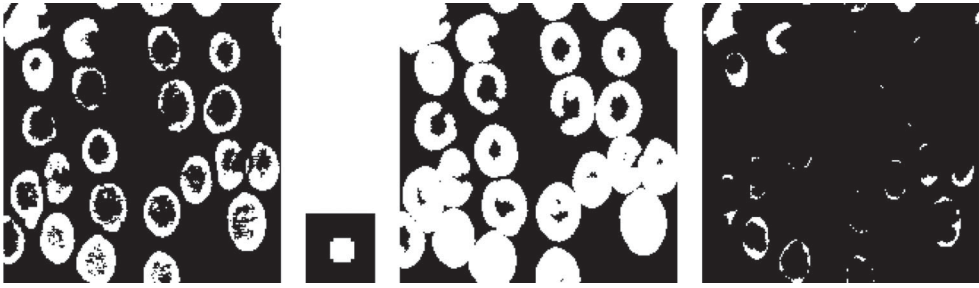
Figure 1. From left to right: binary image, structuring element, dilation, erosion.
