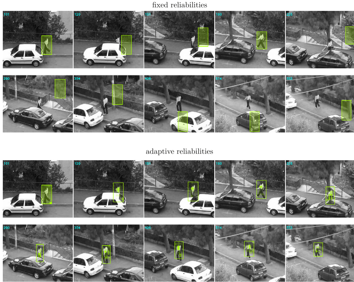
Fig. 7. Sample tracking results with the superimposed reliability maps. First two lines, reliabilities are fixed; last two lines, reliabilities are adapted depending on the context. From the given results, it can be easily seen that adaptive multi-cue integration boosts the accuracy of the tracking process.
