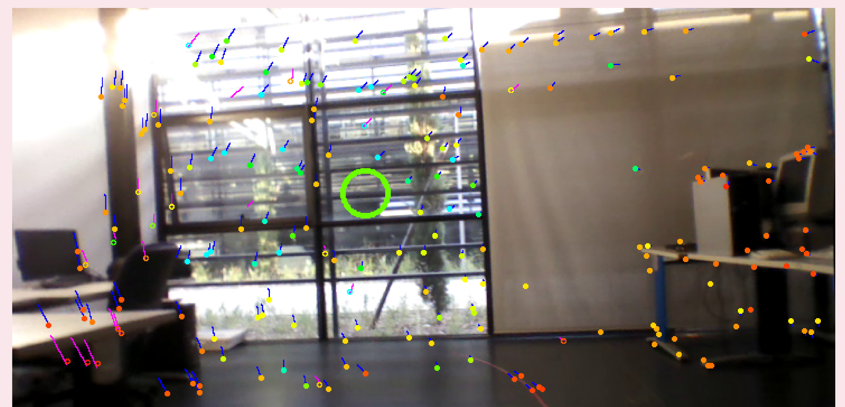
Imperfect sparse 3D reconstructions: A path through a window is planned because of too few correspondences
